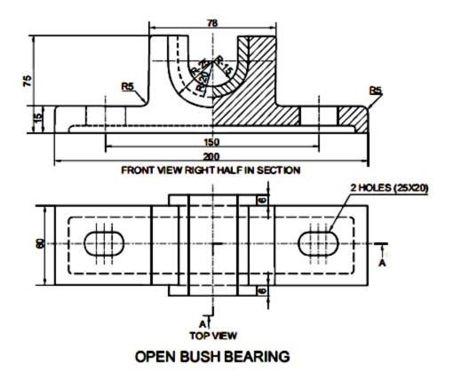
2. The Fig shows the assembly of Bushed Bearing. Dis-assemble the parts, and draw orthographic views of the following parts to scale 1:1, keeping same position:
