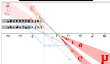
In the figure, images of black letters in a thin convex lens of focal length f are shown in red. Selected rays are shown for letters E, I and K in blue, green and orange, respectively. Note that E (at 2f) has an equal-size, real and inverted image; I (at f) has its image at infinity; and K (at f/2) has a double-size, virtual and upright image.
