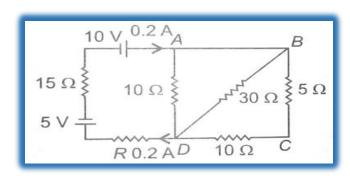
Hints: -equivalent resistance between B and D is  $10\Omega$ . It means 0.2 A of
