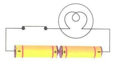
The bulb in the circuit is not glowing because the two cells are not connected properly.
