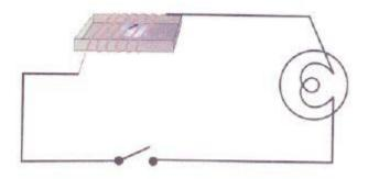
No. The given circuit does not have any current source. In the absence of current, the wire does not behave as a magnet and hence, the compass needle will not show any deflection.
