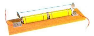
One of the reasons may be that the rubber band used in the cell holder may not be tight enough to keep the two cells in contact with each other. If the cells are not in proper contact with each
