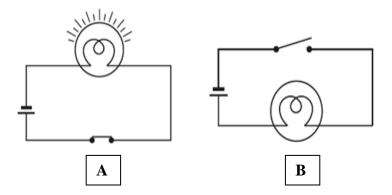
(Hint: A: Closed circuit: When the switch is in the 'ON position, the circuit from the positive terminal of the battery to the negative terminal is complete. The circuit is said to be closed. B: Open circuit: When the switch is in the 'OFF' position, the circuit is incomplete. It is said to be open.)
