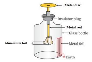
At the top, the metal rod enters in a metallic cup or disc. The bottom of the rod and the metal leaf are enclosed in a glass box for protection. When the disc of the electroscope is touched with a charged ebonite or glass rod, the metal leaves open out or diverge. The extent of divergence
