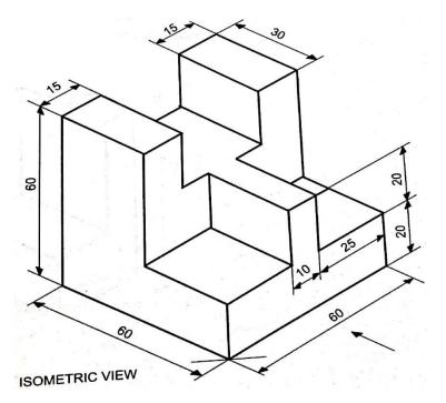
4. Draw to scale 1:1 the front view, top view and side view of the given machine block.
