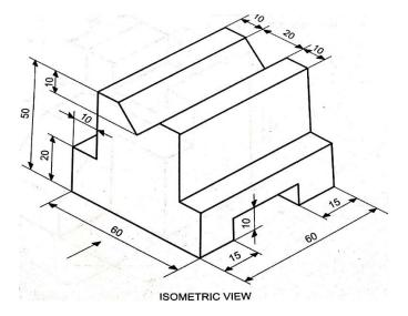
6. Draw to scale 1:1 the front view, top view and side view of the given machine block.
