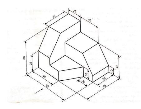
2. Draw to scale 1:1 the front view, top view and side view of the given machine block.
