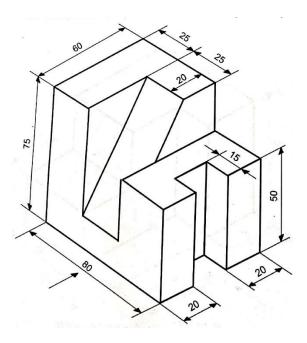
5. Draw to scale 1:1 the front view, top view and side view of the given machine block.
