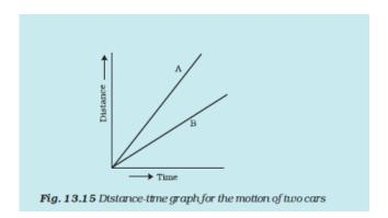
Ans. Vehicle A is moving faster than vehicle B. Greater the slope of distance- time graph , higher is the speed.
