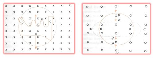
Hints: -(a)The wire is expanding to form a circle, which means that force is acting outwards on each part of wire because of magnetic field (acting in the downwards direction). The direction of induced current should be such that it will produce magnetic field in upward direction (towards the reader). Hence force on wire will be towards inward direction, i.e. induced current is flowing in anticlockwise direction in the loop from cbad.
