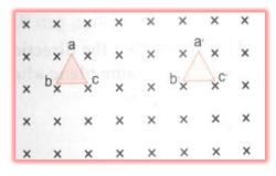
Ans: - change in magnetic flux through wire loop is zero, hence no current.
