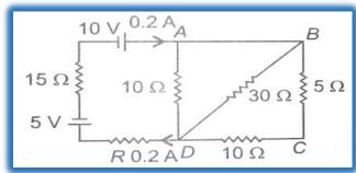
Hints: -equivalent resistance between B and D is  $10\Omega$ . It means 0.2 A of current is divided in to two equal parts of 0.1 A.
