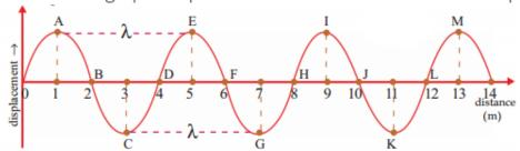
a) In the figure, which are the points of the highest displacement (amplitude)?
