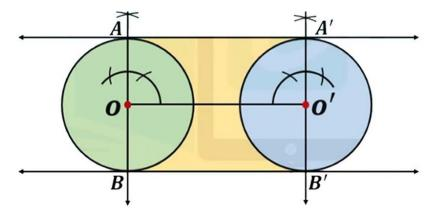
5. Hint: Draw two unequal circles with given diametre touching each other in A,draw the common tangent and transversal.
